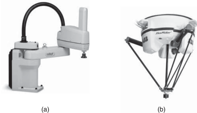
Figure 7.21 SCARA and delta robots are examples of non-Cartesian mechanisms. (a) SCARA robot. Copyright © 2015, Adept Technology, Inc. (Reproduced by permission of Adept Technology, Inc.) [8]. (b) Delta robot (Reproduced by permission of ABB Corp.) [7]
