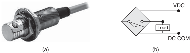
Figure 5.15 Inductive proximity sensor and wiring. (a) Inductive proximity sensor (Courtesy of Rockwell Automation, Inc.) [18]. (b) Three-wire N.O. proximity sensor wired to a load (input card of a motion controller)
